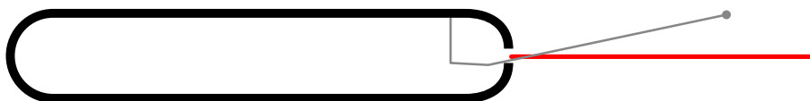
Figure 8.11: Example solution for a target that is unreachable when using the LineGoal. Due to link geometries and joint limits, the second joint of the endoscope is below the opening, requiring the first link to be tilted. The line that the root of the endoscope (circle) should be on is marked in red.
