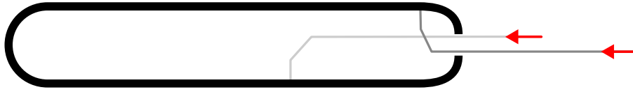
Figure 8.12: Illustration of the alignment objective, constraining the orientation of a link along an axis
