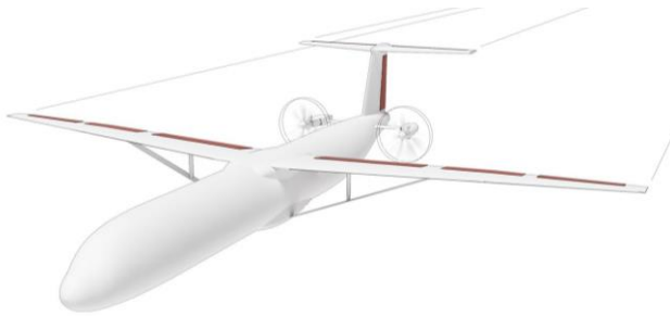
Figure 23: High aspect ratio, strut-braced wing
