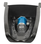
FIG. 11: Suction rib [EU CS2-HLFC-WIN [5]]
