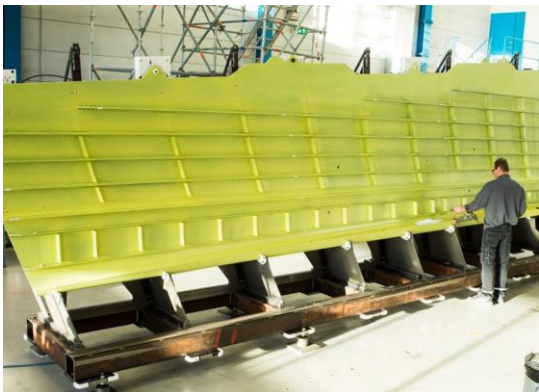
Figure 24: SAAB “Blade” upper wing cover with integrated leading edge (Clean Sky)
