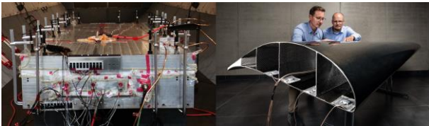
FIG. 13: Multi spar flap [BAB-VPH 2.0] [6],
