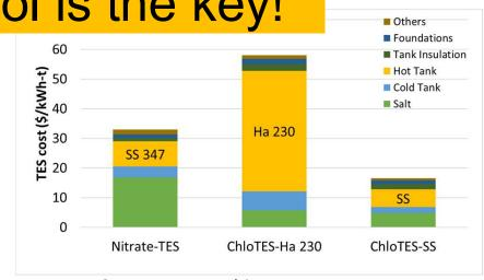
Nitrate-TES cost: 20-33 \$/kWh<sub>th</sub> Chloride-TES with Ha 230 hot tank: 58\$/kWh<sub>th</sub> Estimated Chloride-TES with SS hot tank: ~15\$/kWh<sub>th</sub>
