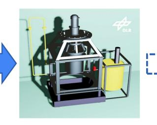
Upscaling with ~100 kg salt: salt purification and corrosion control loop tests, structural materials selection (TRL 4-5)
