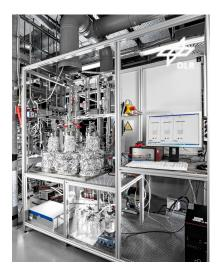
Materials research with <1 kg salt: corrosion control, structural materials pre-selection, ... (TRL 1-3)
