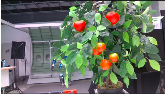
Fig. 5. Identification of tomatoes on the bush with camera and perception algorithm.
