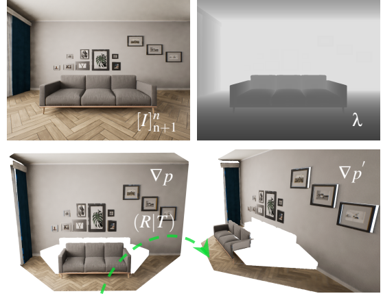
Figure 4: Point Cloud Repositioning: The point cloud \nabla p can be extracted from the original image [I]_{n+1}^n and disparity map \lambda . A new perspective virtual point cloud \nabla p' can be generated by translational and rotational shift (R | T) of \nabla p .
