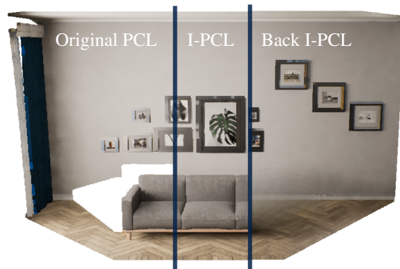
Figure 1: Rendered Point Cloud of 3D Scene with Occlusion, Non-Occlusion and Reconstructed Background: The original point cloud (PCL), on the left, contains white areas which convey the occlusion problem. The center illustrates the result of the inpainted point cloud (I-PCL) reconstructed using our D-LaMa model. The sofa can be hidden by combining PCL and I-PCL. The reconstructed backside is demonstrated on the right.
