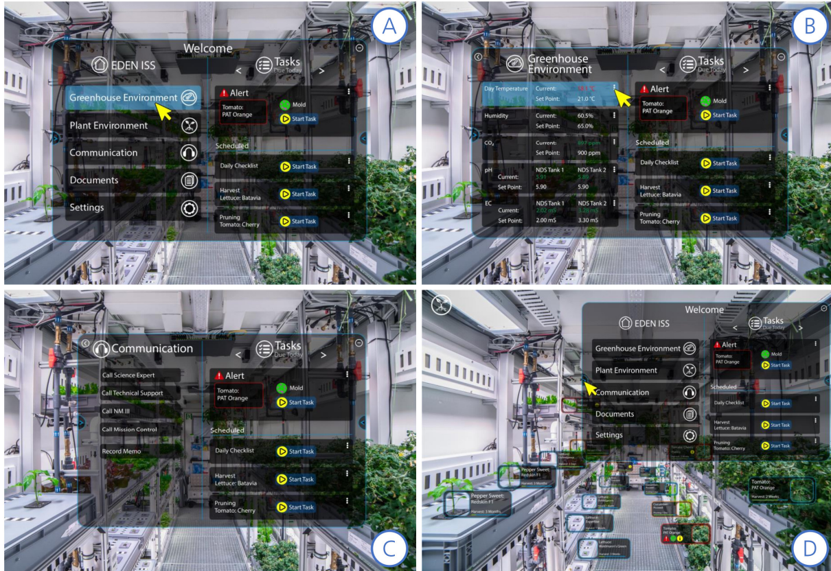
Figure C.1: Concept of the menu and submenus of the ARCHIE 2 augmented reality interface used inside the EDEN ISS greenhouse in Antarctica: (A) Home Screen and Tasks menu; (B) Greenhouse Environment submenu; (C) Communication submenu; (D) Plant Environment mode turned on. The yellow mouse pointer only illustrates a selection action on the interface (not part of the prototype). [91] Photo credits: Hanno Müller.
