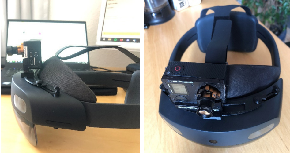
Figure 6.2: Mobile plant health visualizer consisting of a University of Florida Spectral Imager (modified GoPro Hero 4 Black) mounted onto a Microsoft HoloLens 2. [193]
