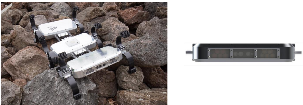
Figure 2: SCOUT rover traversing rocky terrain (left) and rendering of one of the outer modules with integrated lighting system and RGB-D camera (right)
