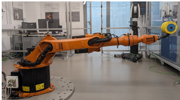
Fig. 7: Experiment setup with KUKA KR16 and laser tracker. Laser probe is attached to the 16kg load facing the laser tracker in the background.
