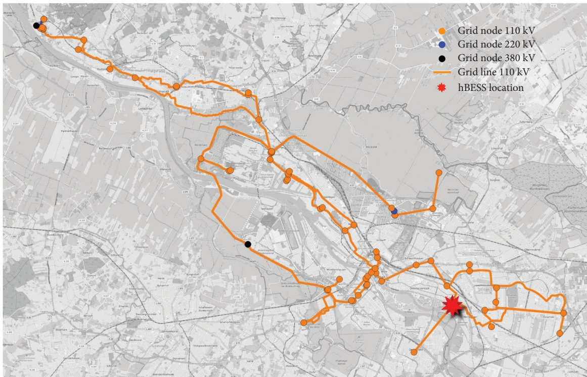
FIGURE 1: The modelled power grid of the German city of Bremen illustrating the nodes and edges for each grid level considered as well as the hBESS location (please note: only 110 kV power lines are visible at this scale). Reference: own illustration. hBESS, hybrid battery energy storage system.
