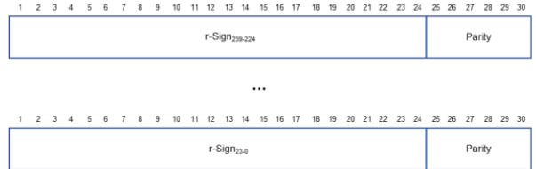
Figure 5: R-Mode TESLA ECDSA signature r-value with type "10" (l-value analogue with type "11", not shown)
