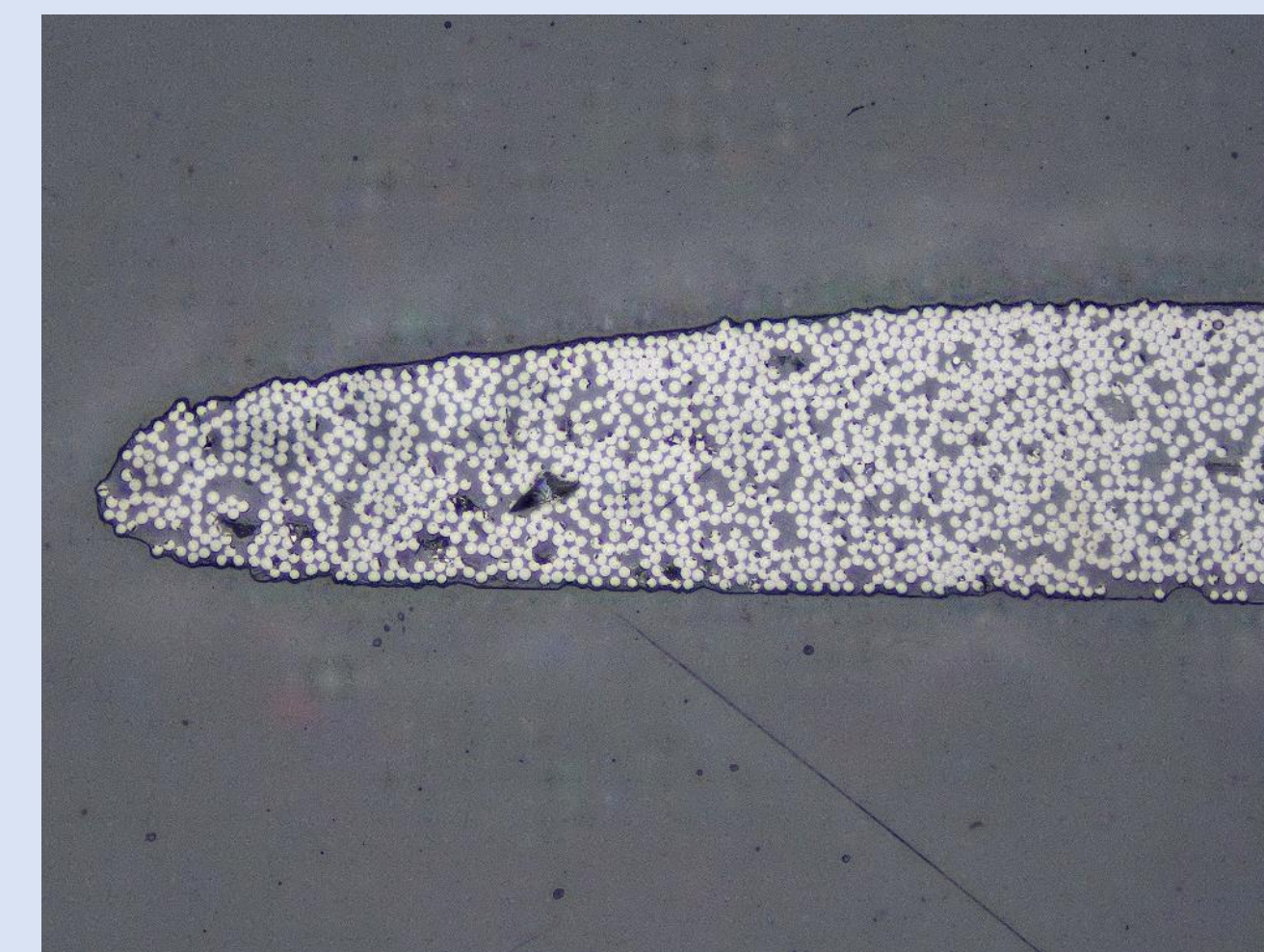
Figure 8. Typical tape edge cross-section view after processing
