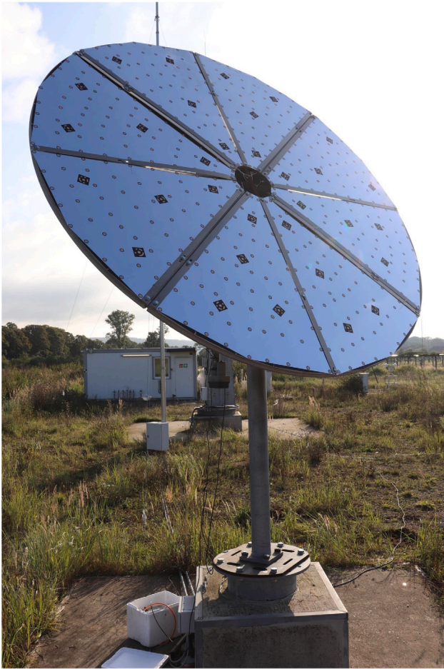
Fig. 8. Front view of the assembled concrete heliostat on the HeliTep at the solar tower Jülich (Germany).
