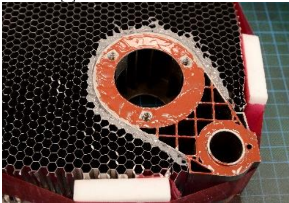
Figure 3: Insert with RTV glue applied on facesheet interface
