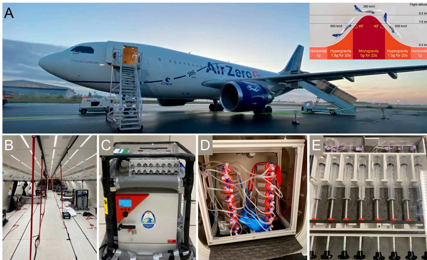
Figure 2. Highlights from a parabolic flight campaign (PFC). (A) The Airbus A310 AirZeroG aircraft operated by Novespace for the 41st DLR PFC at Bordeaux-Mérignac Airport, France. Insert shows the gravitational changes with the time sequence of a parabola; (B) inside of the AirZeroG aircraft allowing installation of several in-flight-operable experimental racks; (C) example of a PFC flight rack with an incubator and injection unit; (D) inner part of the incubator showing installation of tissue culture flasks harboring living human cells. Each flask is connected to the injection unit by a separate tubing; (E) the injection unit is used to fix the cells, as shown during maintenance and experimental setup.
