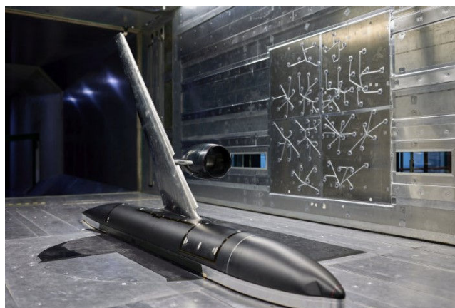
Figure 16 – Microphone wall array mounted on the sidewall of the closed test section [21]
