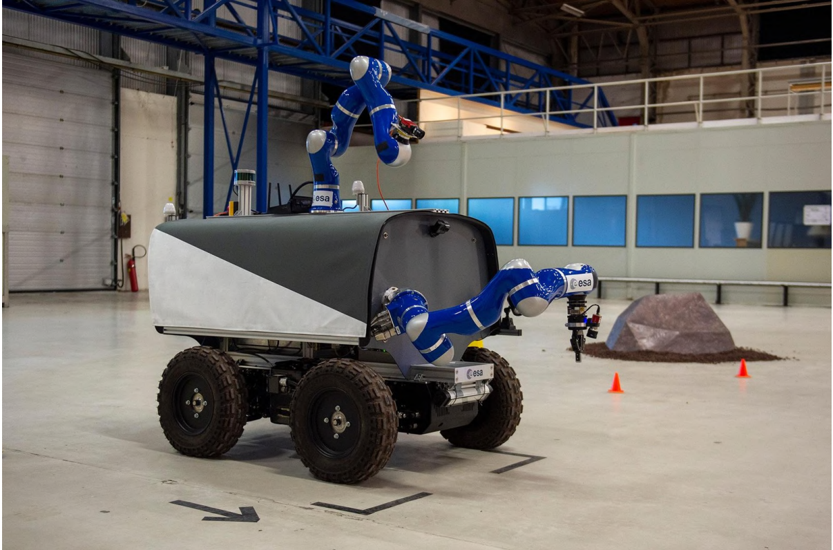
Figure 4.2: Image of interact rover used in the Surface Avatar. (Krueger et al. 2020a)
