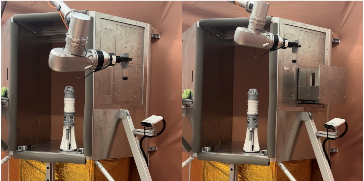
Figure 6.9: Sample Stowage Device in use during a dry run test. The mission was simulating the return of a Sample Tube to the Sample Stowage Device using TINA.
