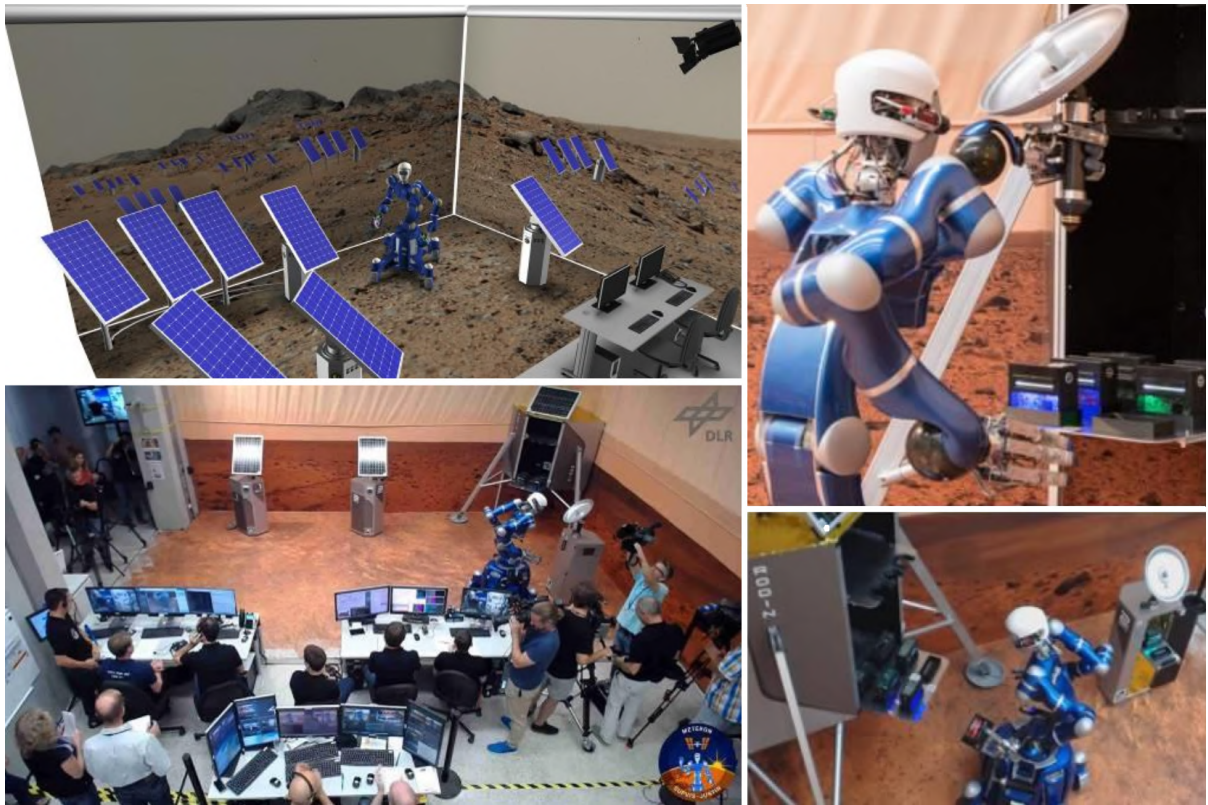
Figure 2.7: The top-left image shows the METERON configuration of SOLEX, simulating a Martian environment, with the presence of Rollin' Justin and the SPUs. The bottom-left image shows the advanced SOLEX setup with the inclusion of the Lander in the right corner. The two images on the right show the SOLEX lander with its cargo bay storing the CUs and the satellite dish on the tray. (Bayer et al. 2019)
