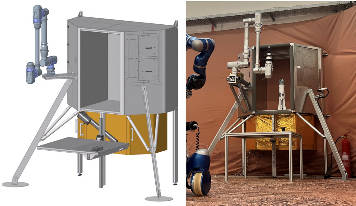
Figure 6.18: On the left: representation of the Lander with the Electronics Bay in metallic gold. On the right: The Lander during the execution of the Seismometer protocol.
