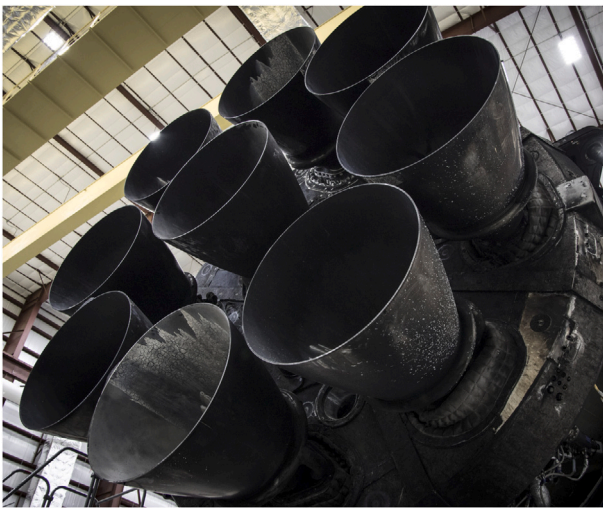
Fig. 10. Illustration of cluster arrangement where 8 peripheral nozzles surround a central nozzle (SpaceX Photos, CC0, via Wikimedia Commons).
