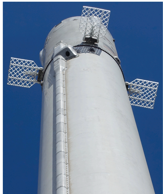
Fig. 11. Deployed grid fins on a Falcon 9 booster (Steve Jurvetson, CC BY 2.0, via Wikimedia Commons).
