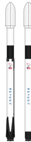
Fig. 4. Illustration of the Falcon 9 launch system showing the re-usable variant directly next to the expendable model (Lucabon based on work of Markus Sáynevirta and Craigboy and Reessi), CC BY-SA 4.0, via Wikimedia Commons.
