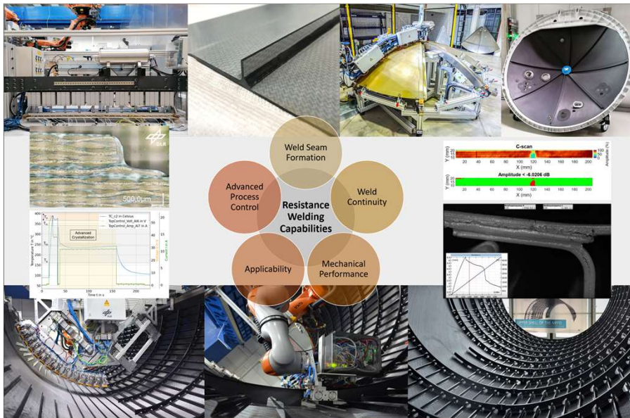
Excerpt on the capabilities of the static resistance welding process at test bench level, as well as applied in the automated assembly of fiber composite structures in an exemplary representation of the thermoplastic rear pressure bulkhead and the Multifunctional Fuselage Demonstrator (MFFD) upper shell.
