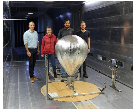
Fig. 6 A 1.0 m test sphere in the DNW Low Speed Wind Tunnel.
