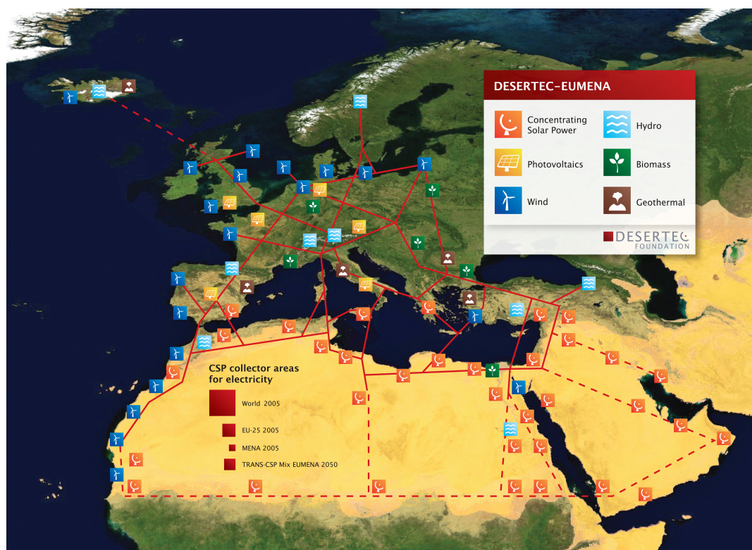
Fig. 1.1.: Outline of a possible infrastructure for sustainable power supply in Europe, the Middle East and North Africa (EU-MENA). Squares indicate required area for solar collectors to meet the energy demand as of 2005. The "TRANS-CSP Mix EUMENA 2050" is the prospected area (120x120km) to realize DESERTEC by 2050 according to the TRANS-CSP scenario developed by DLR, covering 17% of european electricity demand. Source: DESERTEC Foundation. CC BY-SA 2.5
