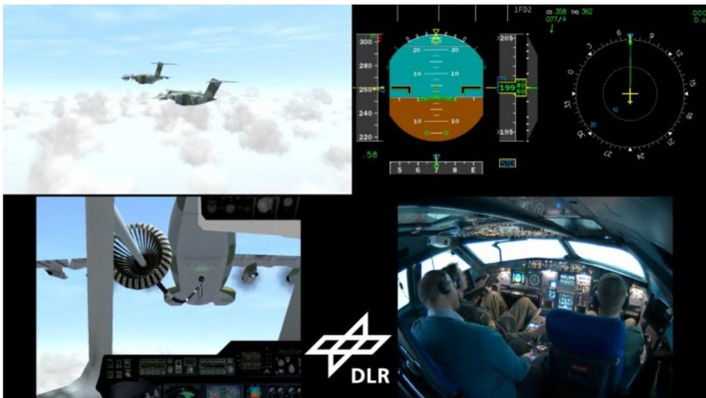
Figure 11 – Simulator tests with FMTA as receiver in the AVES simulator with A400M pilots
