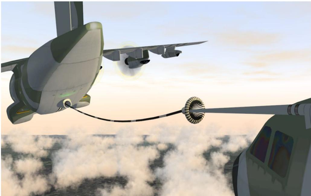
Figure 4 – Simulated centerline refuelling with two FMTA
