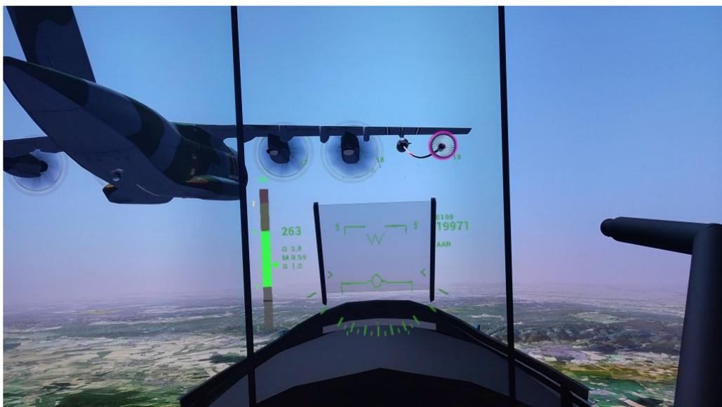
Figure 9 – Pilot assistance for fighter air-to-air refuelling using HoloLens 2
