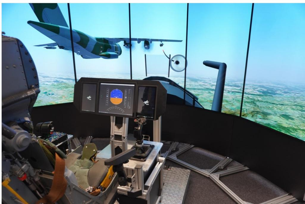
Figure 8 – Military Air Vehicle Simulator - Fast Integration Testbed (MARS-FIT) at DLR in Manching
