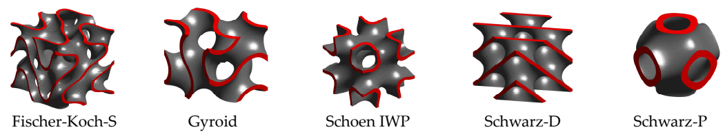
Figure 3. Unit cells of thickened cubic TPMS structures ( t_{\text{ref}} = 0 ) with a void fraction of 80% and a specific surface of 100 \text{ m}^2/\text{m}^3 .
