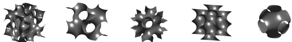
Figure 1. Different TPMS structures in a unit cell, from left to right: Fischer-Koch-S, Gyroid, Schoen IWP, Schwarz-D, and Schwarz-P.
