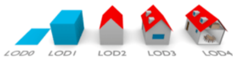
Figure 2: The five different LoDs for 3D Building Models in CityGML (Biljecki et al. 2016). Licensed under CC BY-NC-ND 4.0 DEED.
