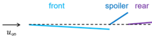
Figure 10. Sample visualisation for a VLM spoiler configuration with additional deflections of the aerodynamic boxes in front of and behind the spoiler
