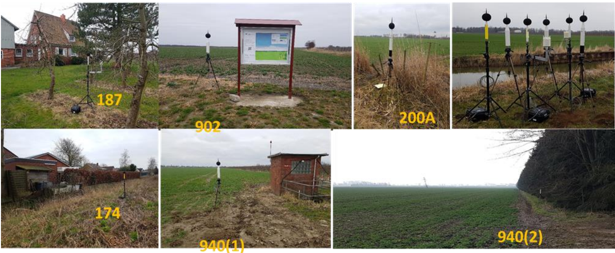
Figure 3: View on the single microphone sites during the measurement in march 2021. At the beginning of the measurements all six microphones were placed together to intercalibrate them in terms of sound pressure level as well as their internal clocks (upper right frame).
