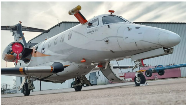
Fig. 3 Embraer Phenom 300 flight test aircraft: prototype aircraft with all modifications for the SENS4ICE North America flight test campaign (credit Embraer)
