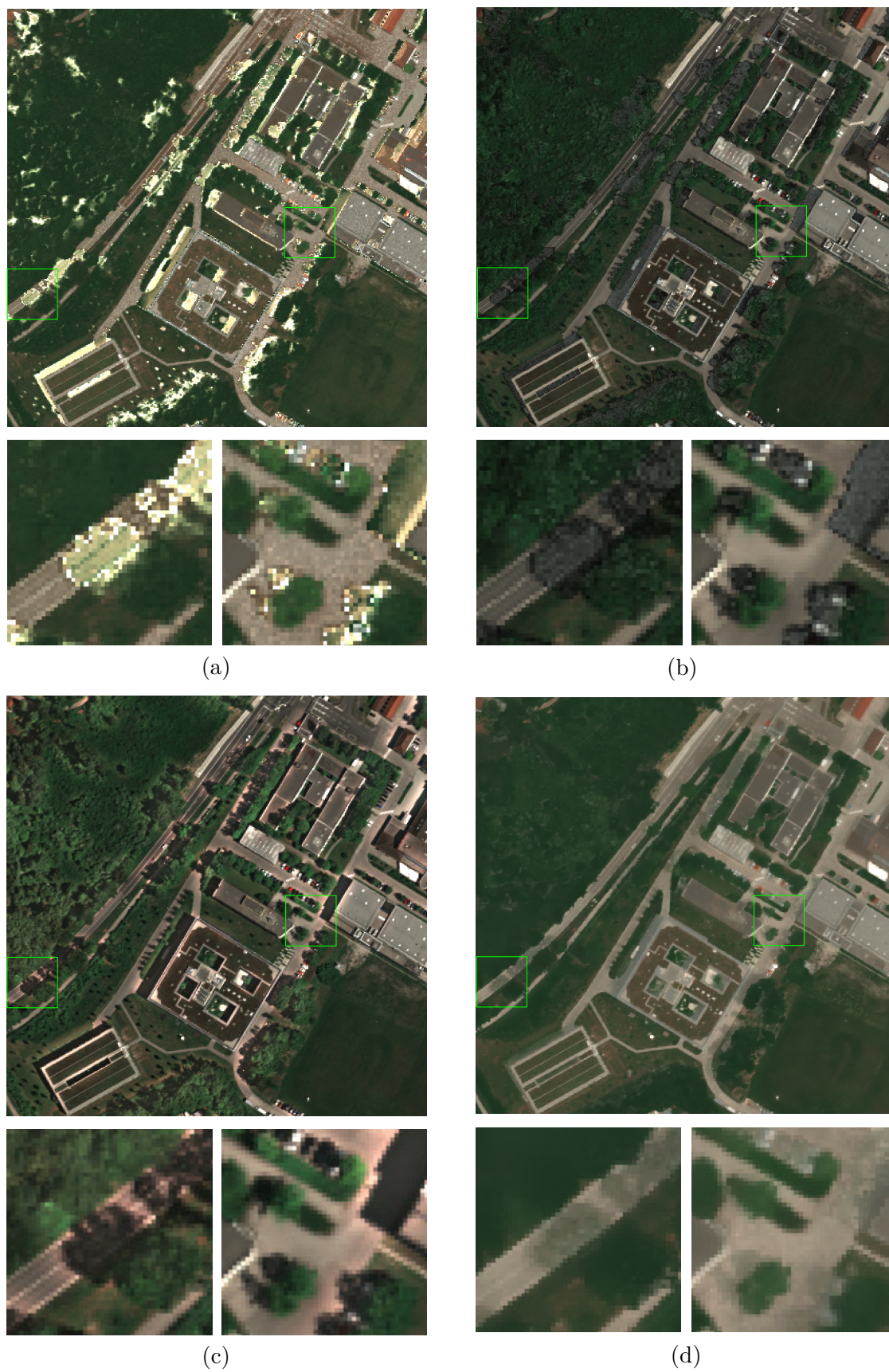
Figure 5.50: Comparison of shadow removal methods using hyperspectral imagery with a size of 400-by-400 pixels shown in true color composite. (a) SLMM (b) NUEM, (c) MEXPO, and (d) S3AM.
