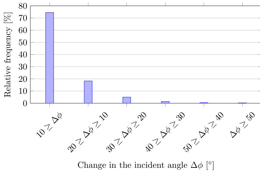
Figure 3.6: Relative frequencies of changes in incident angles exceeding a certain difference in the incident angle \Delta\phi based on secondly data obtained at the STJ.
