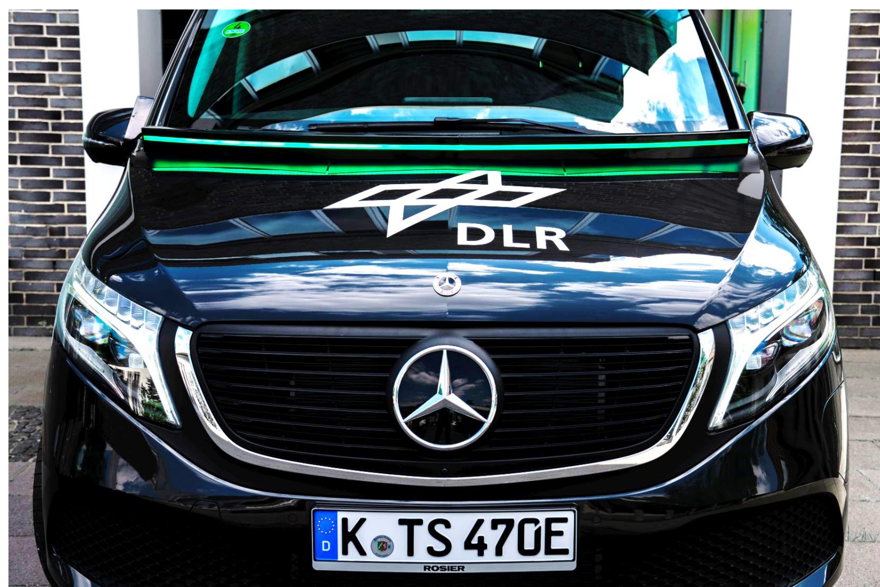
Fig. 2: One of DLR's cooperative automated vehicles (CAV) with a green bar as external human-machine interface (eHMI).
