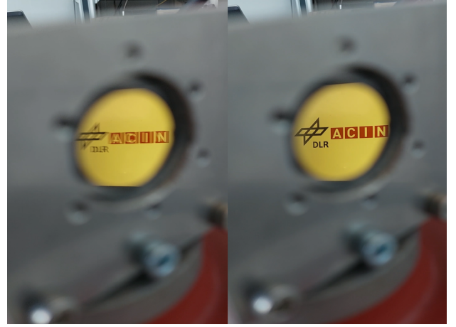
Fig. 8: Qualitative comparison of open-loop (left) and closed-loop (right) jitter under external vibration using two logos reflected from an external monitor on the mirror surface. Displayed is the FSM3000 with 0.45 gRMS.
