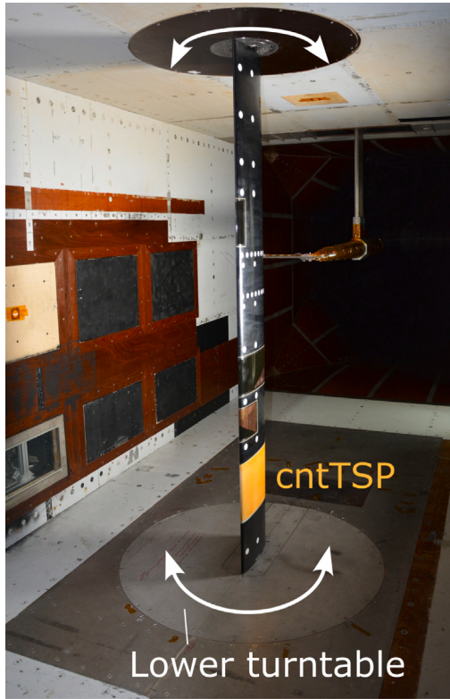
Fig. 1. Downstream view (in direction of wind tunnel flow) of the cntTSP-coated wind tunnel model in the test section.
