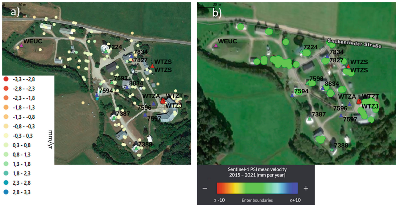
Fig. 1 PSInSAR LOS velocities at the Wettzell Observatory from two different processings of Sentinel 1A/1B data, descending orbit 095. (a) EGMS level 2A products, 2015/02 to 2021/12, (b) German ground
