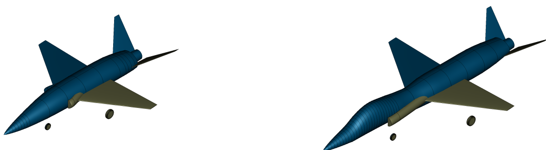
(a) Atreus , designed for a sustained load factor of 7 g, carrying 2 ARMs in an internal payload bay
