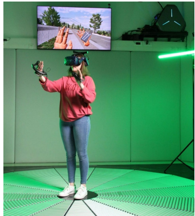
Fig. 1 The pedestrian simulator of the MoSAIC
