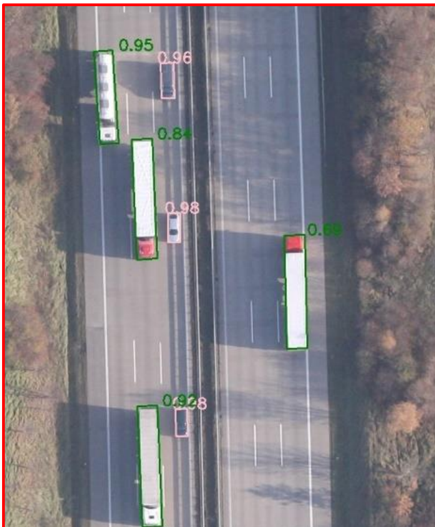
Figure 34. Vehicle detection and classification dataset with confidence scores assigned to each vehicle
