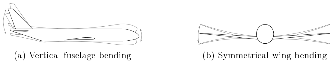
Figure 2.2: Typical structural mode shapes.
