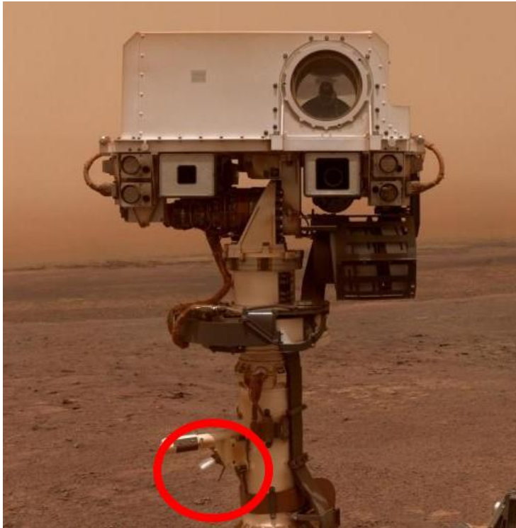
Figure 1: REMS-H is located in the boom of Curiosity's mast. Credit: NASA/JPL-Caltech/MSSS
