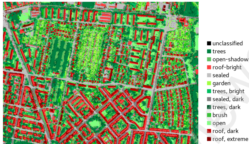
Figure 2: Self-adaptive classification of the Gohlis district in Leipzig, Germany. 24 clusters formed by the Imalys process "fabric" method were combined into 13 classes (legend). The classification were based on aerial photographs and elevation model.
