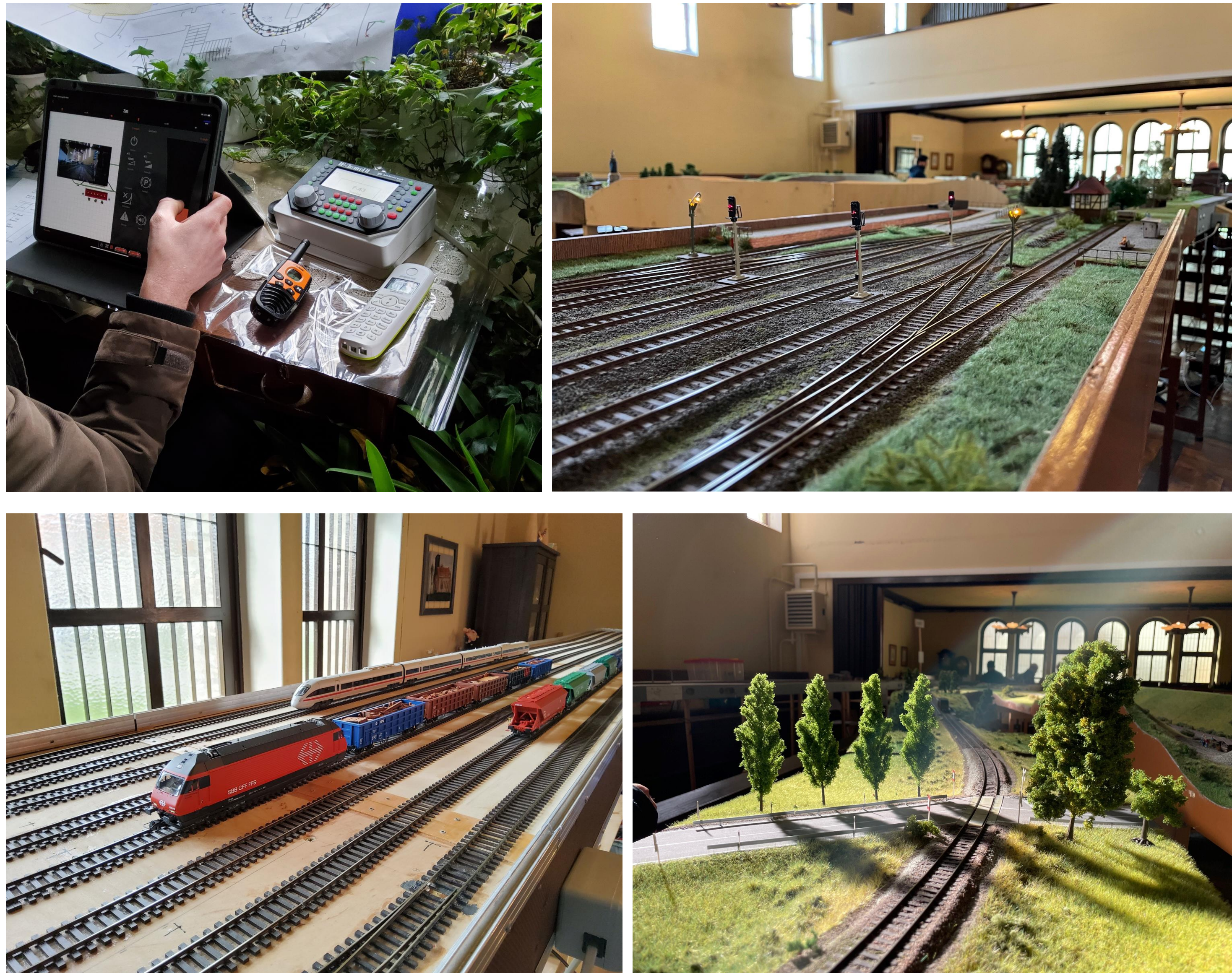
Fig. 1. Remote Operator workplace (upper left) separate from the railway model layout (right). Lower left: Test locomotive (Re460 series with integrated video camera) in the staging yard.
