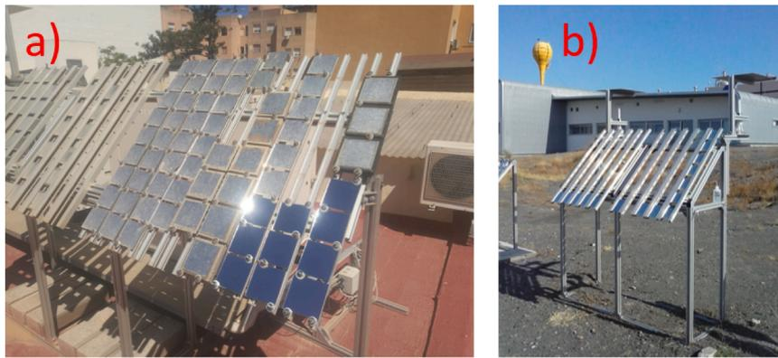
Fig. 12. Outdoor exposure of reflector samples at two different sites: a) Almería and b) Tabernas (PSA, owned by CIEMAT).
