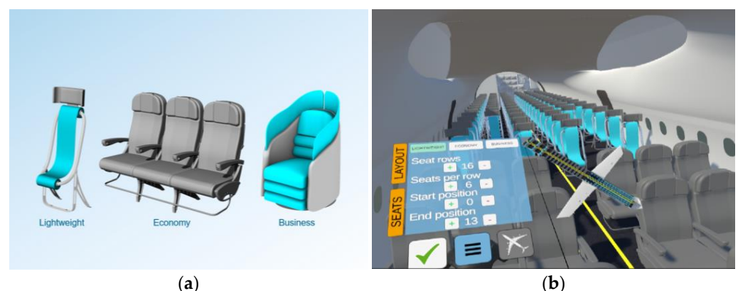
Figure 2. (a) Available seat types (from left to right): half standing lightweight seat, economy seat, and business seat. (b) User interface of the VR application from the perspective of a participant.
