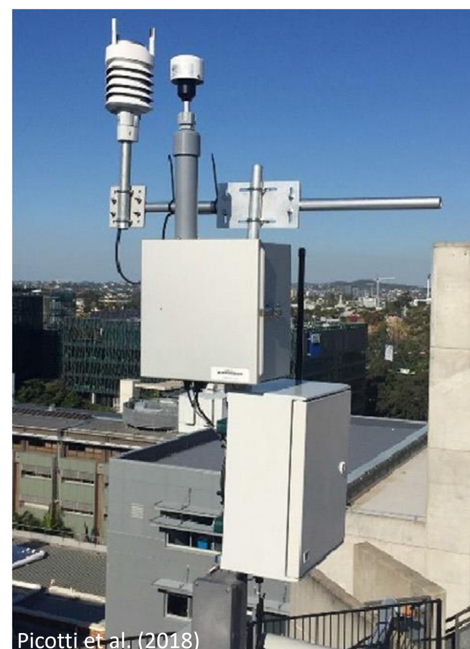
Fig. 4: Category 4 – Protinus 1000 Dust Monitor Station
