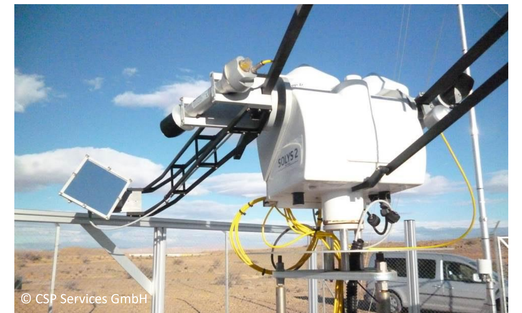
Fig. 5: Category 3 – TraCS instrument installed on Kipp & Zonen sun tracker Solys 2
