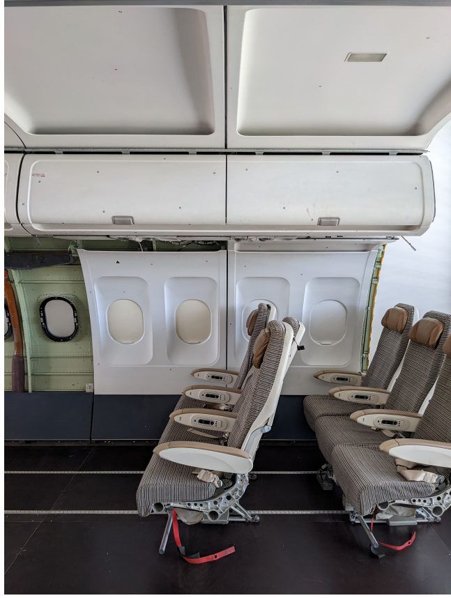
Figure 6.2.19.: Section of OHSC and two sidewall and ceiling panels (cabin mock-up at the DLR Institute of System Architectures in Aeronautics)
