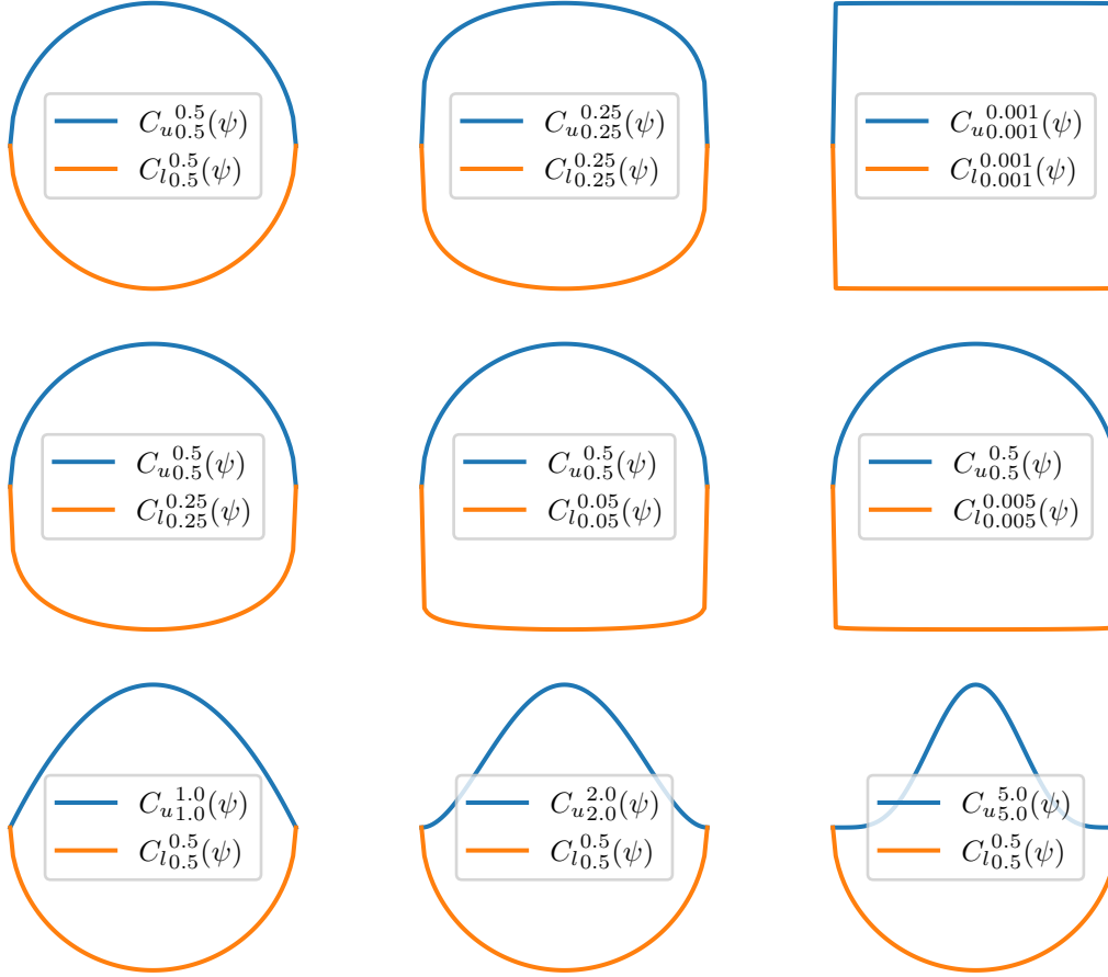
Figure 4.1.5.: CST representations for different fuselage profiles (after [Kul08])
