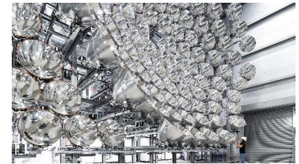
Synlight® Solar Simulator („Largest artificial sun“)
