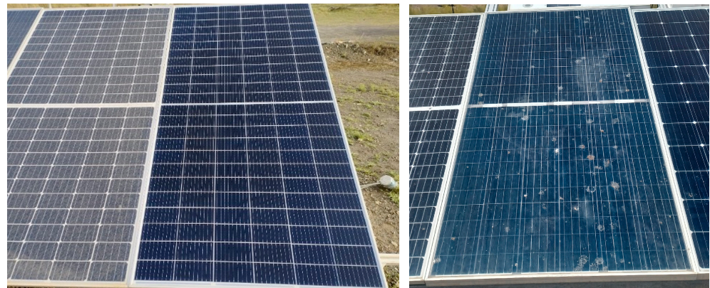
Figure 1. Illustrating two different soiling types. Left: two modules next to each other. The left one is soiled with dust and the right one is cleaned. This soiling is classified as homogeneous. The accumulation of dust is slightly stronger only in the lower row of cells. Right: Module soiled with bird droppings. This module is considered to be inhomogeneously soiled.
