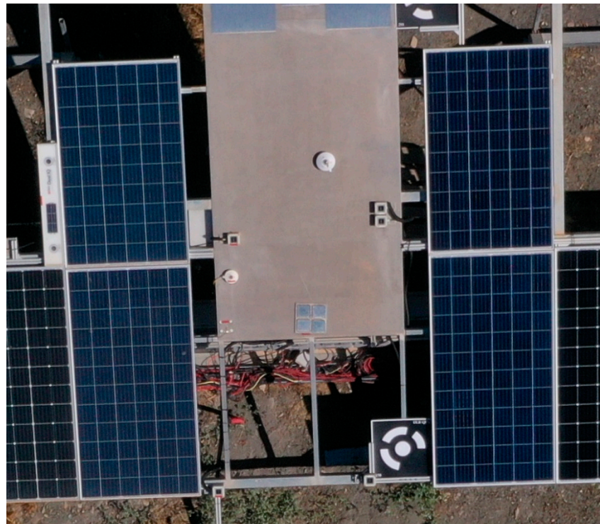
Figure A6. The setup during the second campaign. The modules on the right are both clean. Out of these two, the lower right was used as a clean reference. The lower left module was used as a soiled reference.
