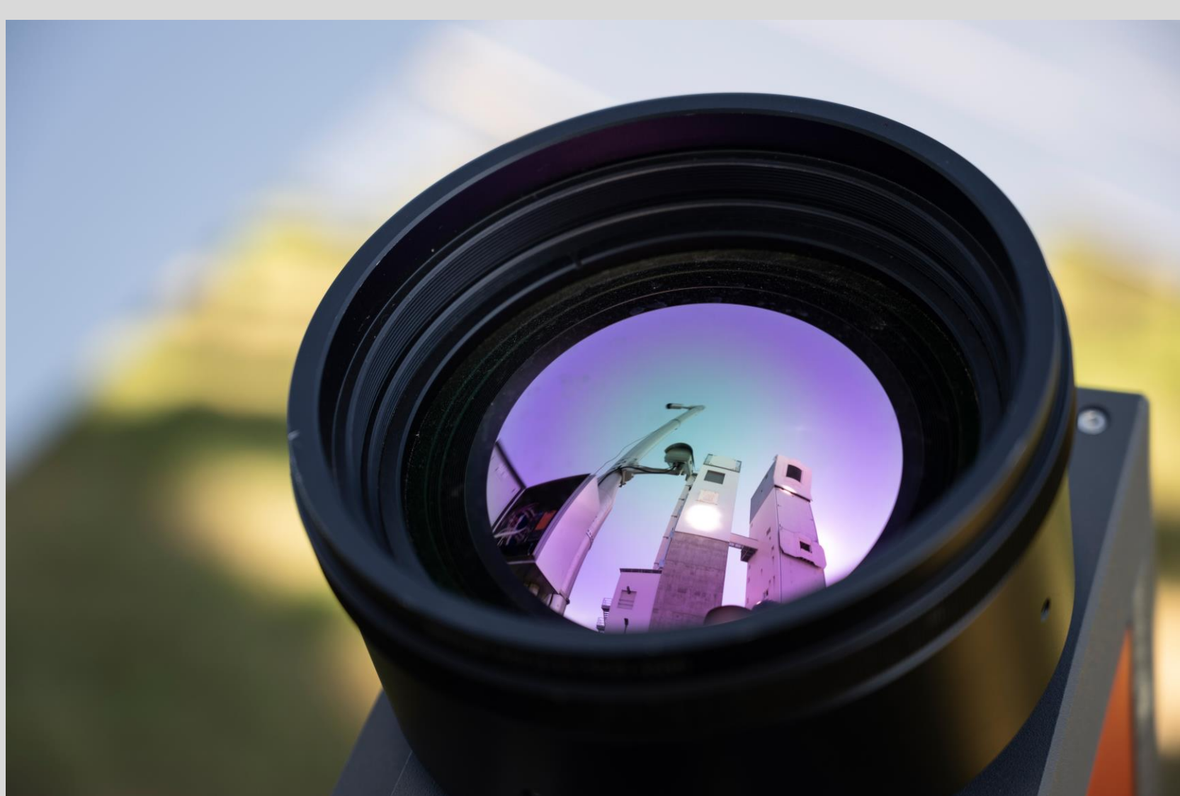
Figure 4: Infrared camera looking at the irradiated receiver
