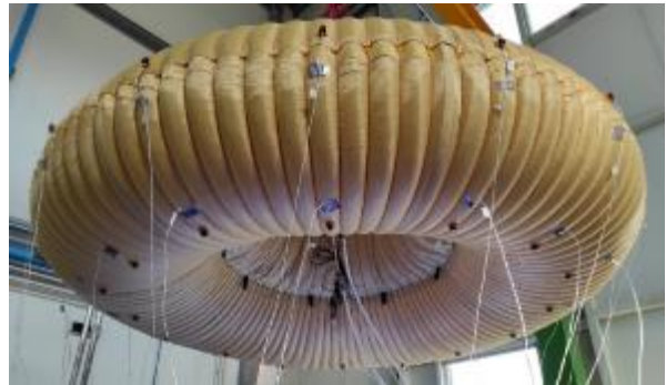
Fig. 21. IS demonstrator under excitation (free-free).
