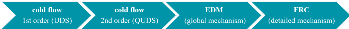
Figure 4.3: ThetaCOM simulation workflow with three stages concerning the reactivity of the flow: cold flow, EDM and FRC, with each stage consisting of two phases, implemented by the use of six subsequent parameter files
