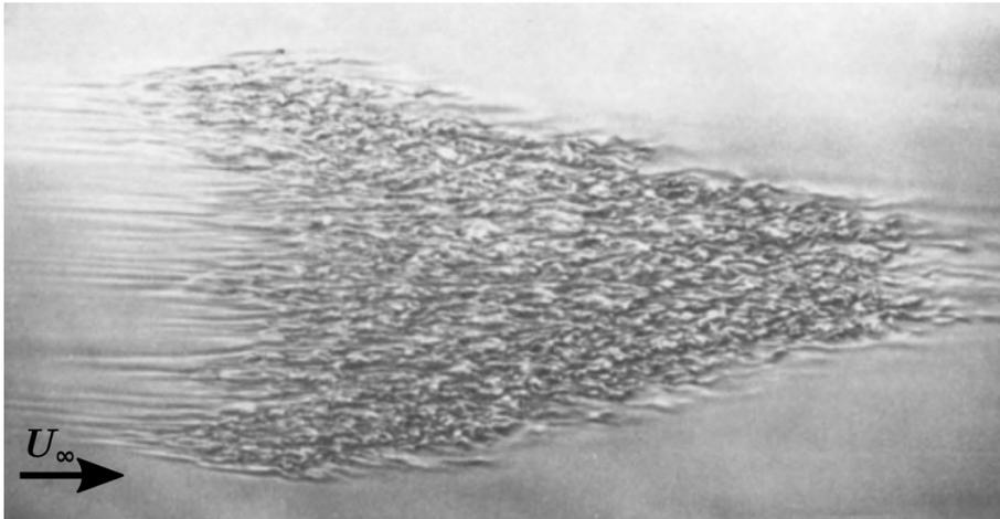
**Figure 1.1:** Visualisation of sublayer streaks of a turbulent spot in water illustrated with the use of aluminium flakes at  $U_\infty = 0.23$  m/s. Adapted from Cantwell et al. [17]. No scale was given by the original authors, but based on the description of the experimental setup, the spanwise extent of the turbulent spot is in the range of several centimetres.
