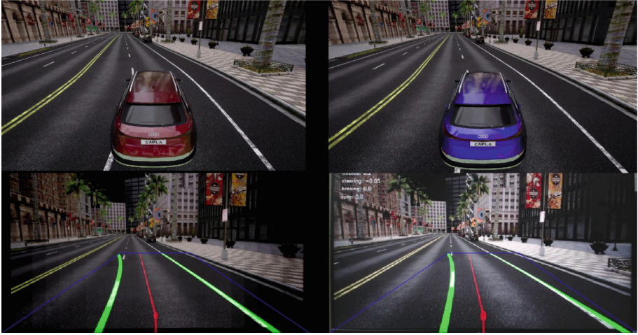
Fig. 10. Footage taken from DS (left) and AMDEV-bed (right). The upper images show the two representations in their respective virtual environment and the lower images are the modelled and actual footage, respectively.
