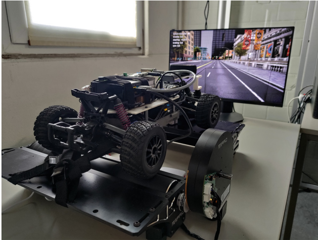
Fig. 4. Image of the miniature ViL testbed setup called AMDEV-bed in an early stage of development. It shows the model car on a roll stand in front of a monitor.
